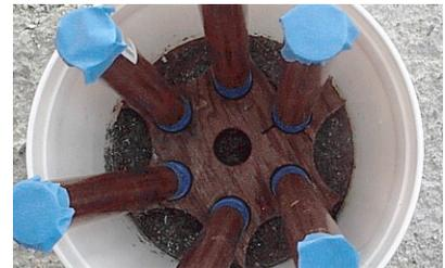
Expediently move the Template 2 down on to the six pipes until it is snugly within the rim of the bucket. Put the top Template 3 onto the top of the pipes and move them until the pipes are parallel. After the resin has hardened, remove the second template and set it aside. This is only used during construction, as I mentioned.
